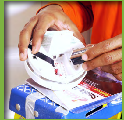
Check smoke alarm batteries every six months to make sure they are working.
